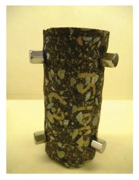
*Figure 10. Test specimen from Maine CCPR project ready for dynamic modulus testing.*
