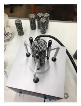
*Figure 8. LVDT stud gluing jig showing custom arms.*
