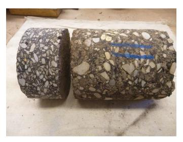
*Figure 5.* Core from FDR project in Edmonton showing a debonded surface layer.
