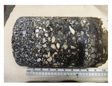
*Figure 2.* Core obtained from FDR project in Delaware.
