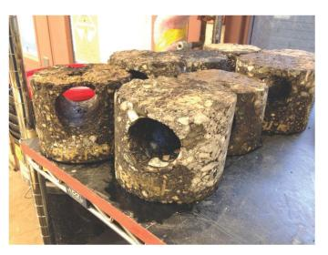
*Figure 7. Field cores from which test specimens were extracted.*
