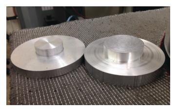
*Figure 9. AMPT testing platens with removable pacer blocks for 38 mm and 50 mm diameter small-scale specimens.*
