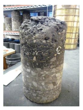
Figure 4. Core from FDR project in Delaware showing missing portion of recycled layer.
