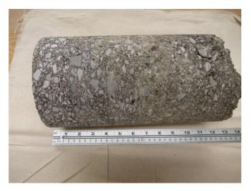
*Figure 3.* Core obtained from CIR project in West Virginia.
