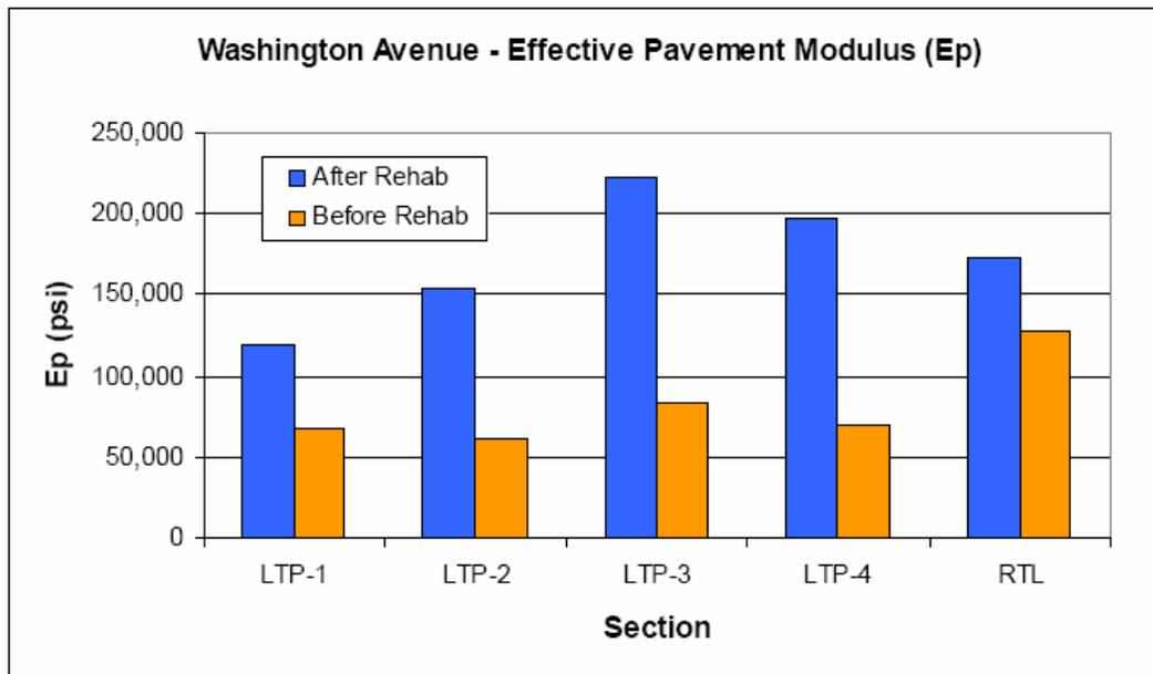
**FIGURE 6 Comparison of effective pavement modulus.**
