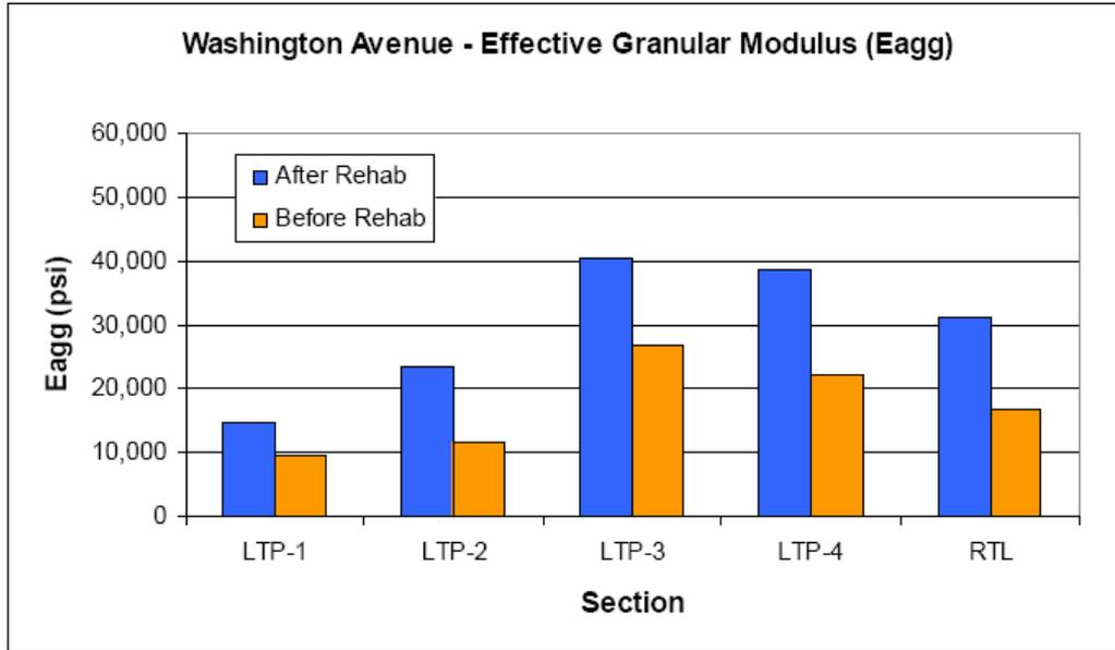
**FIGURE 5 Comparison of the effective granular modulus.**
