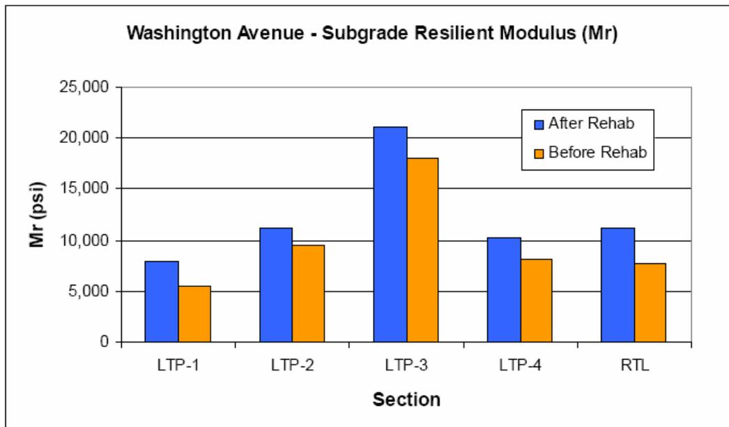
**FIGURE 4 Comparison of the subgrade resilient modulus.**
