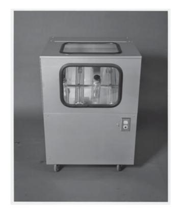
**ABRASION MACHINE - CLOSED**
