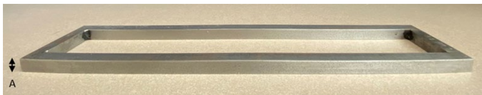
Figure 7 - Side View of Specimen Mold
