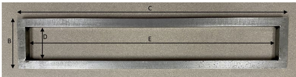
Figure 8 - Top View of Specimen Mold
